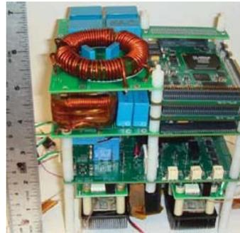
15 kW @ 6.3 kW/l with  $\theta_{jmax} = 250\text{ }^{\circ}\text{C}$
