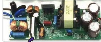
220 W LED driver using Wolfspeed C3M SiC MOSFETs
