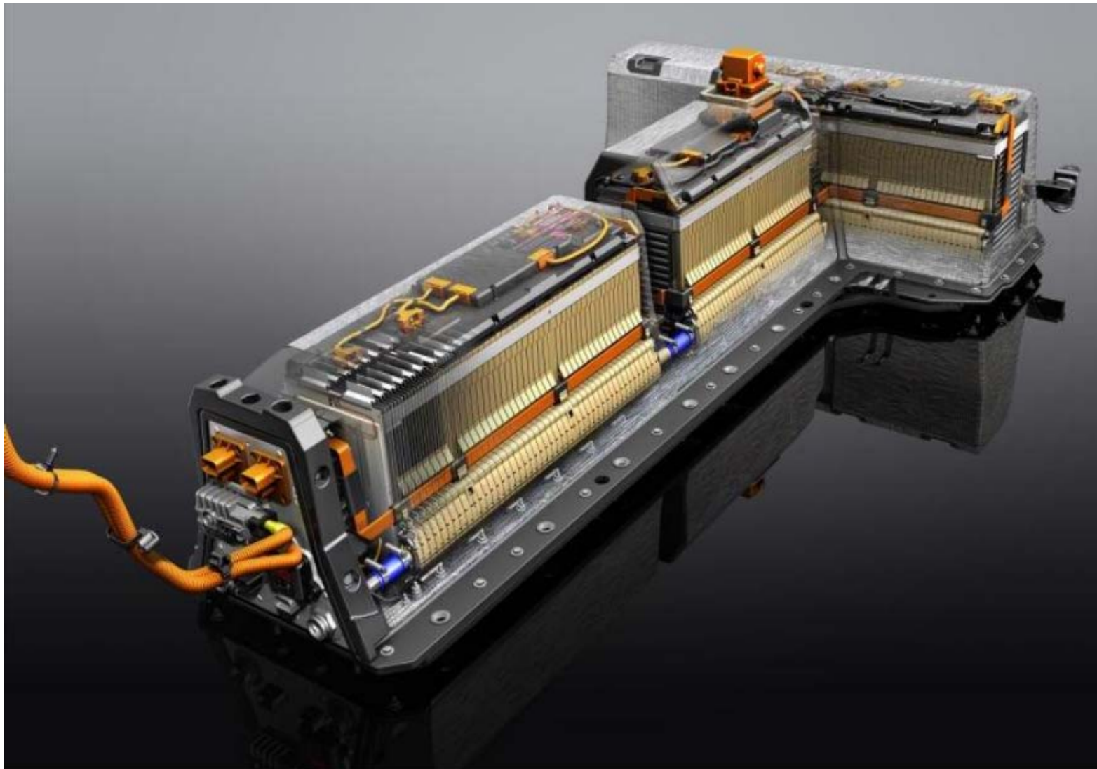
Figure 3.3: The battery pack of the Chevrolet Volt (General Motors, 2010).
