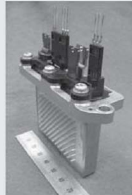
(b) Power module with double-sided direct cooling
